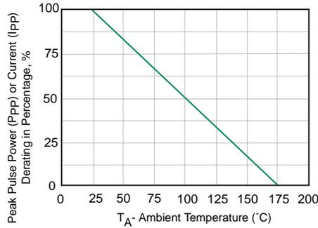
Fig. 2 Pulse Derating Curve
