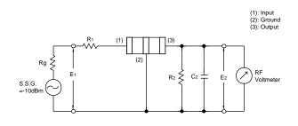
$$\begin{split} Rg &= 50\Omega \quad R_1 = 280\Omega \pm 5\% \quad R_2 = 330\Omega \pm 5\% \\ C_2 &= 10 \pm 2 \text{ pF (Including stray capacitance and Input capacitance of RF Volt Meter)} \\ E_1: S.S.G. \quad S.S.G. Output Voltage \end{split}$$
