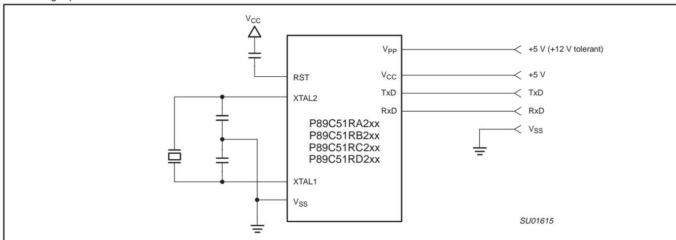
Figure 41. In-System Programming with a Minimum of Pins
