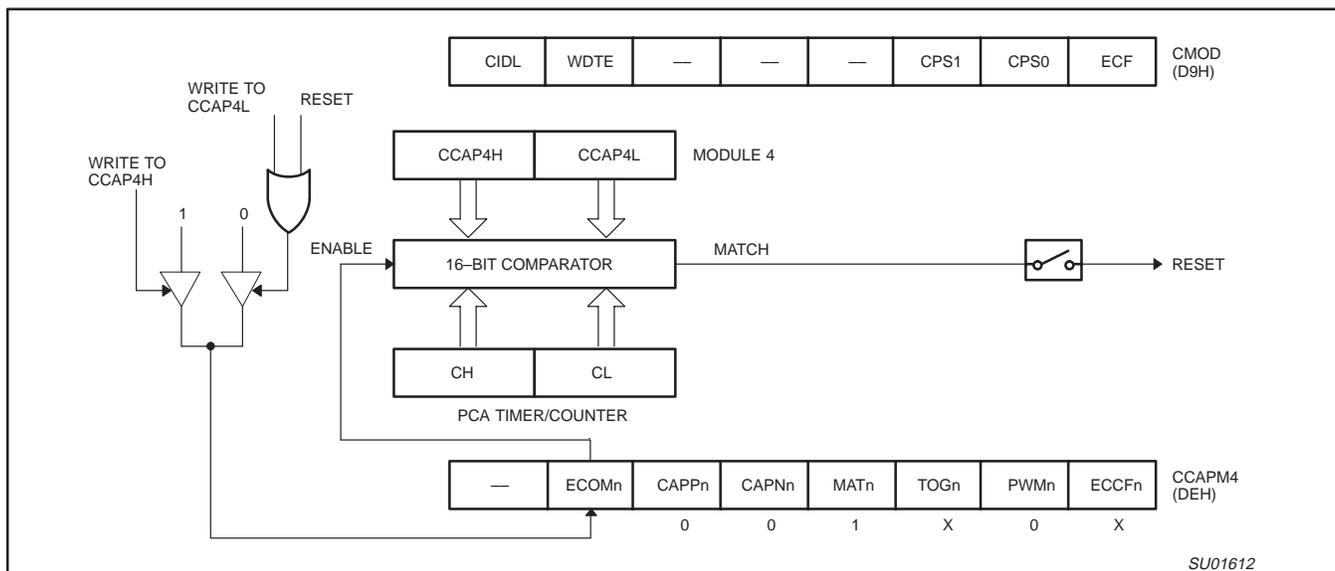
**Figure 36. PCA Watchdog Timer mode (Module 4 only)**
