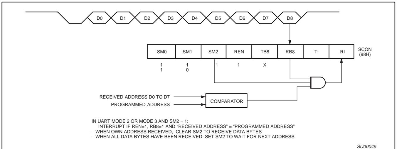
Figure 20. UART Multiprocessor Communication, Automatic Address Recognition
