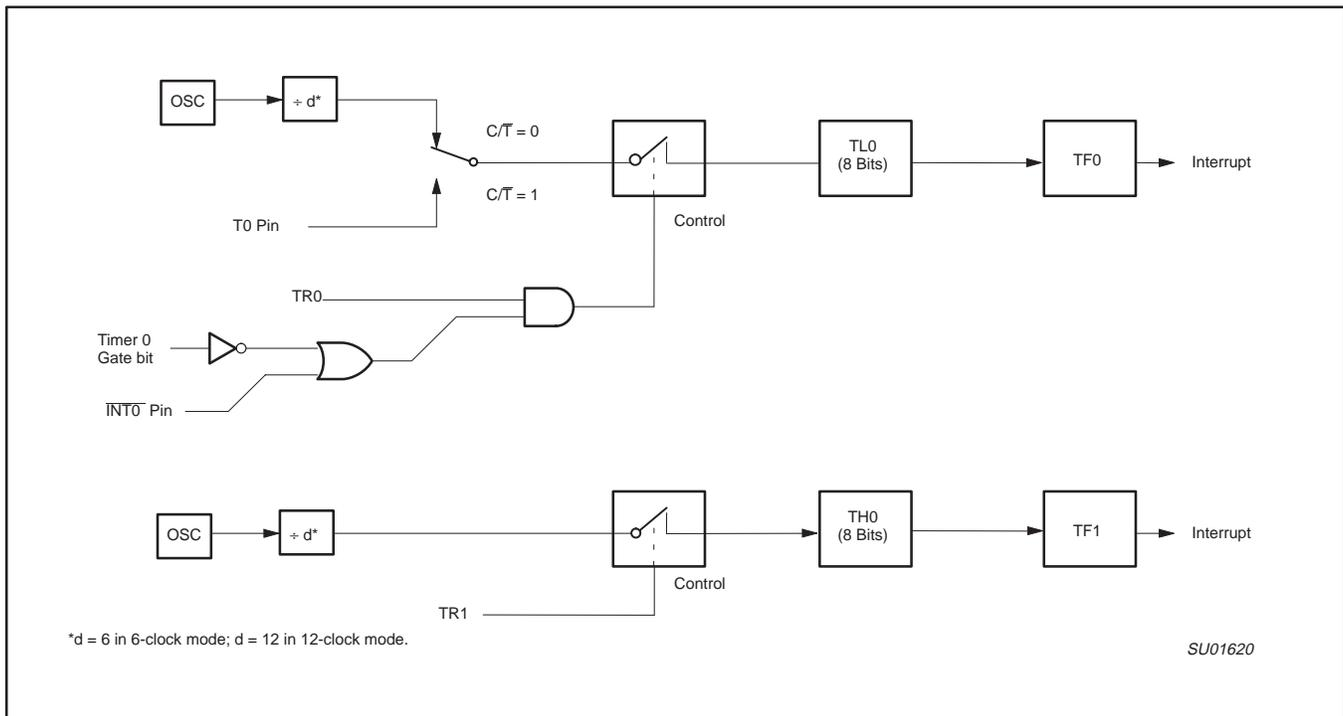
Figure 5. Timer/Counter 0 Mode 3: Two 8-Bit Counters
