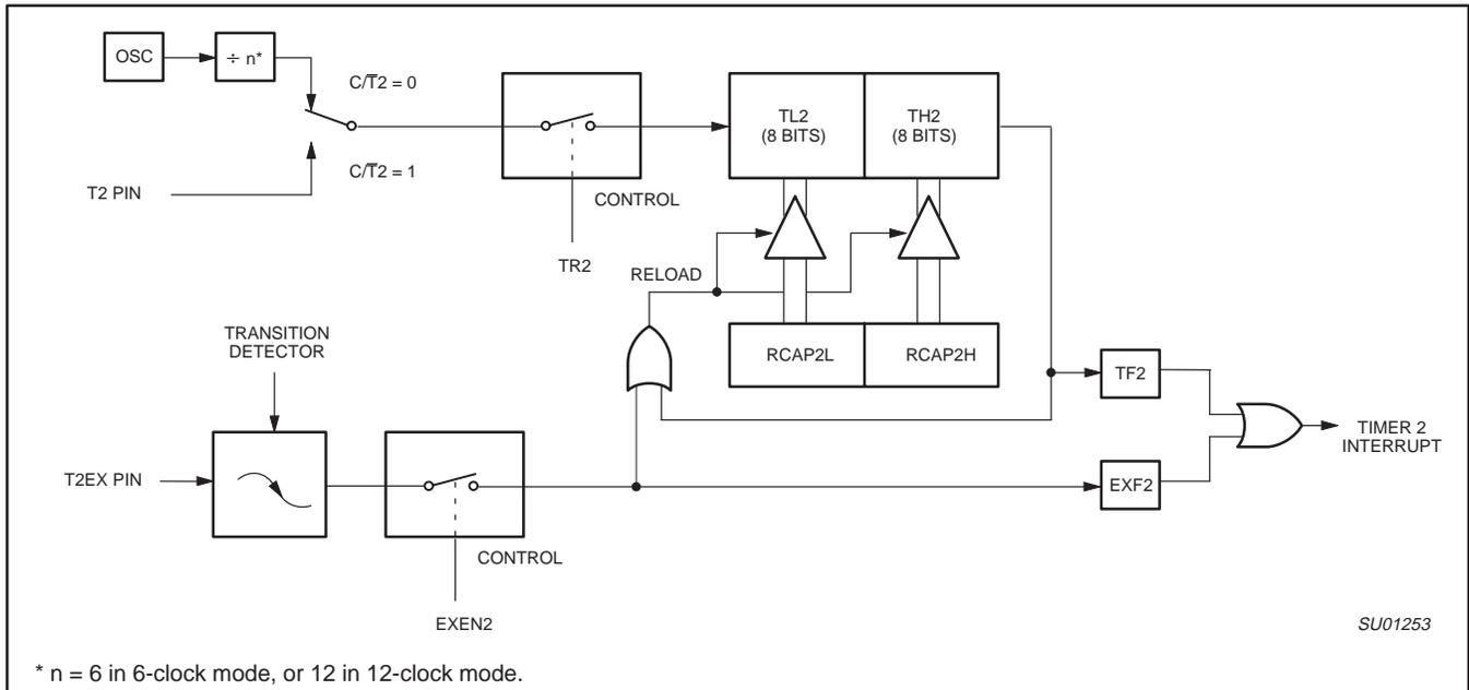
Figure 9. Timer 2 in Auto-Reload Mode (DCEN = 0)
