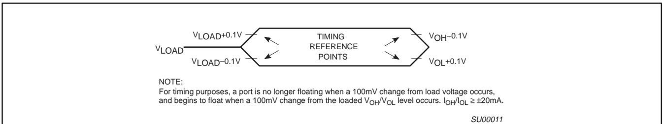
Figure 51. Float Waveform
