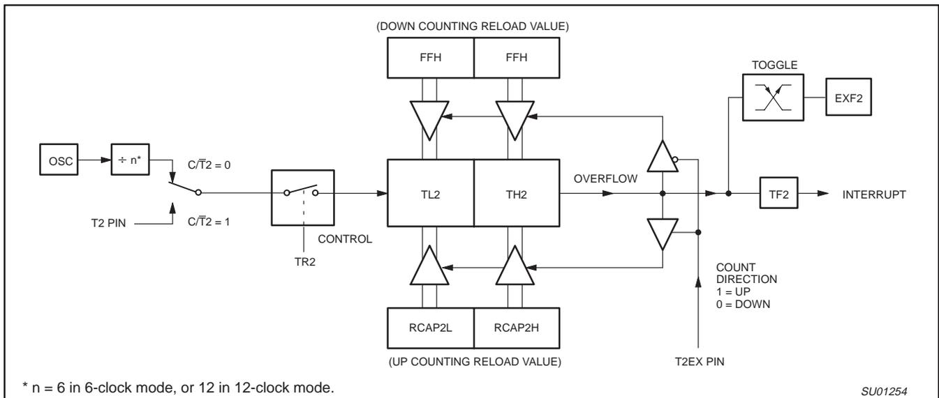
Figure 10. Timer 2 Auto Reload Mode (DCEN = 1)
