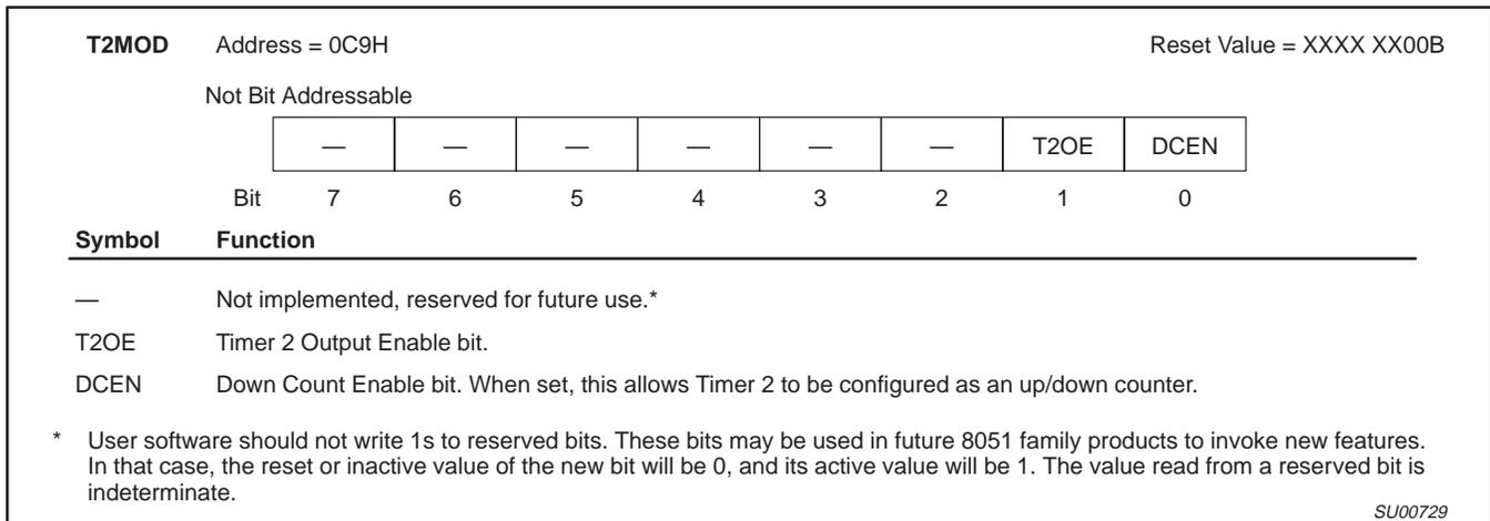
**Figure 8. Timer 2 Mode (T2MOD) Control Register**
