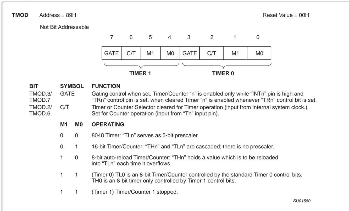
Figure 1. Timer/Counter 0/1 Mode Control (TMOD) Register
