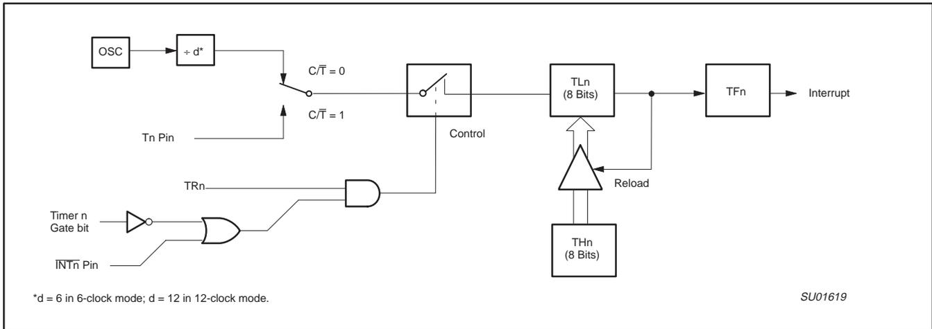
Figure 4. Timer/Counter 0/1 Mode 2: 8-Bit Auto-Reload
