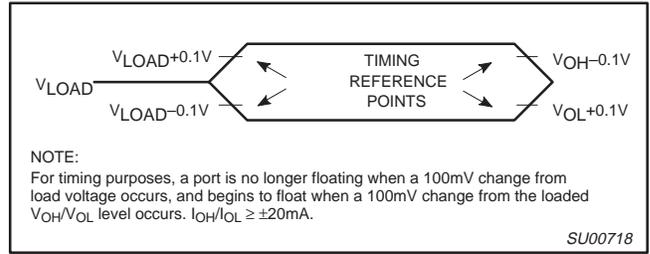
Figure 48. Float Waveform
