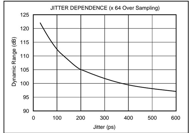
FIGURE 18. Jitter Sensitivity.
