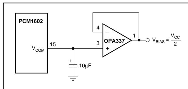
FIGURE 11. Biasing External Circuits Using the V<sub>COM</sub> Pin.
