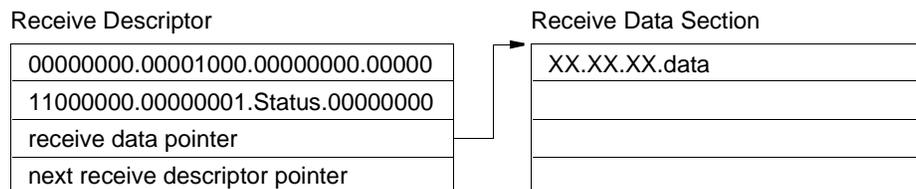
The data bytes are stored into the receive data section according to the Little Endian convention (Intel mode) or Big Endian convention (Motorola mode).
