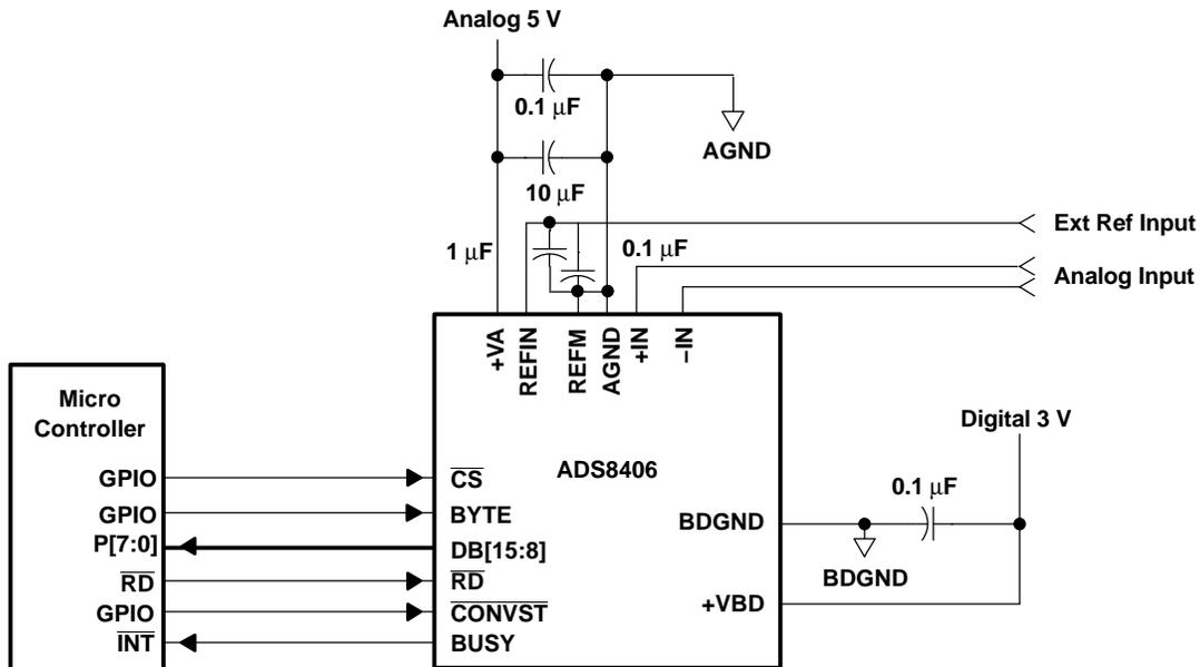
Figure 31. ADS8406 Application Circuitry (using external reference)
