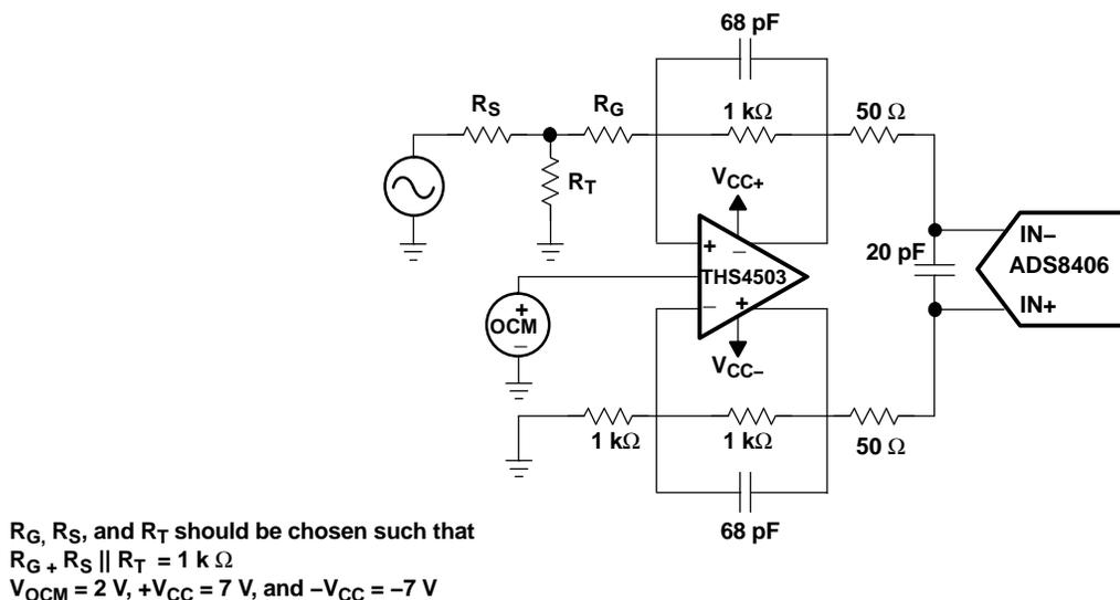
**Figure 33. Using the THS4503 With the ADS8406**
