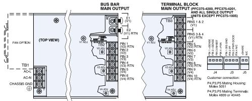
INPUT & OUTPUT CONNECTIONS: 6-32 SCREW TERMINAL ON 0.375" (9.5mm) CENTERS BUS BAR MAIN OUTPUT, E1 & E2, 10-32 SCREW TERMINAL
