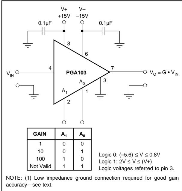
FIGURE 1. Basic Connections.
