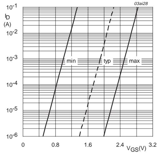
$T_j = 25 \text{ }^{\circ}C; V_{DS} = 5 \text{ V}$
