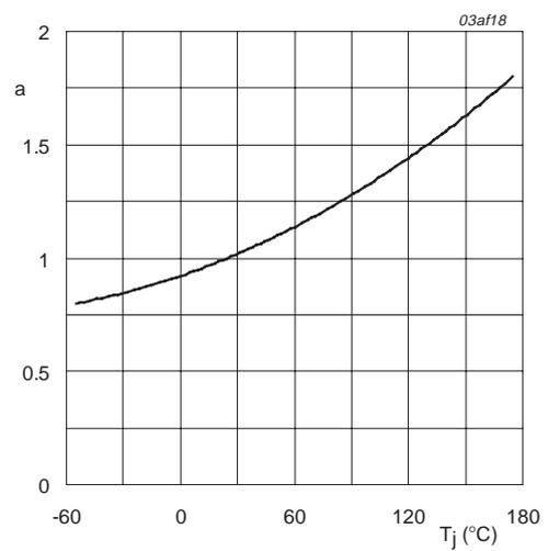
$$a = \frac{R_{DSon}}{R_{DSon(25^\circ\text{C})}}$$
