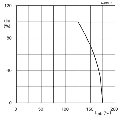
$$I_{der} = \frac{I_D}{I_{D(25^{\circ}C)}} \times 100\%$$
