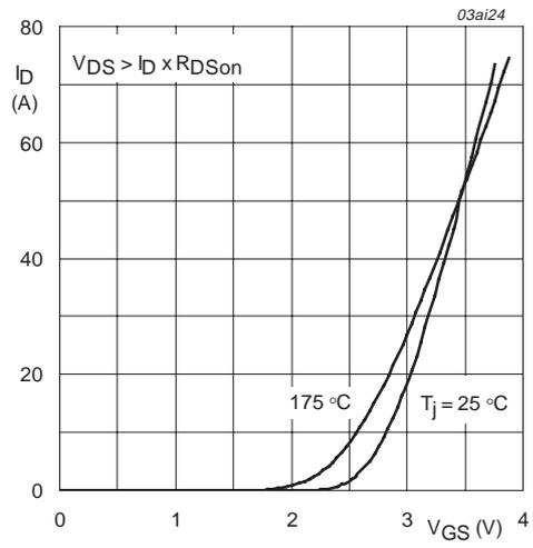
$T_j = 25\text{ }^\circ\text{C}$  and  $175\text{ }^\circ\text{C}$ ;  $V_{DS} > I_D \times R_{DSon}$
