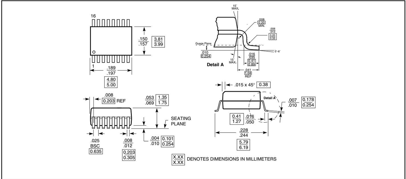
**Packaging Mechanical: 16-Pin SOIC (W)**
