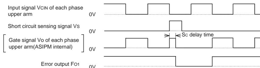
Note : Short circuit protection operation. The protection operates with "Fo" flag and reset on a pulse-by-pulse scheme. The protection by gate shutdown is given only to the IGBT that senses an overload (excluding the IGBT for the "Brake").
