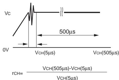
Note ; Ringing happens around the point where the signal output voltage changes state from "analogue" to "data hold" due to test circuit arrangement and instrumental trouble. Therefore, the rate of change is measured at a 5 µs delayed point.
