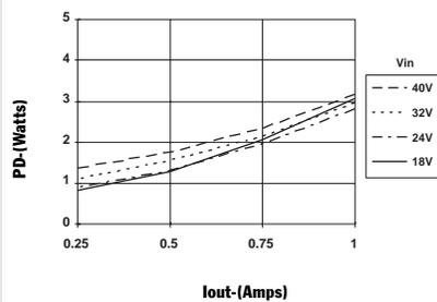
**Note 1:** All data listed in the above graphs, except for derating data, has been developed from actual products tested at 25°C. This data is considered typical data for the DC-DC Converter.
