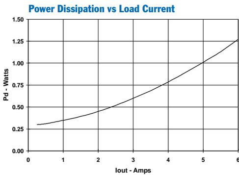
**Note A:** Characteristic data has been developed from actual products tested at 25°C. This data is considered typical data for the Converter.
