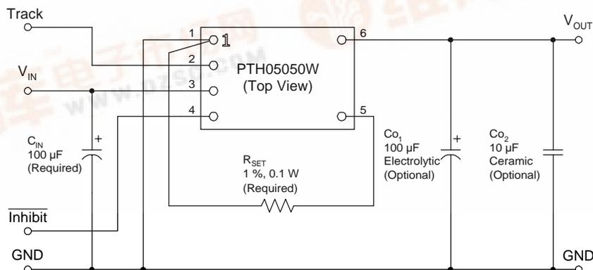
R<sub>set</sub> = Required to set the output voltage to a value higher than 0.8 V. (See spec. table for values)
