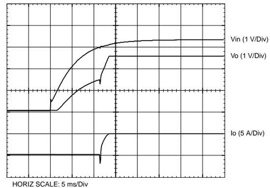
**Figure 3-9; Application Circuit Demonstrating Pre-Bias Startup**
