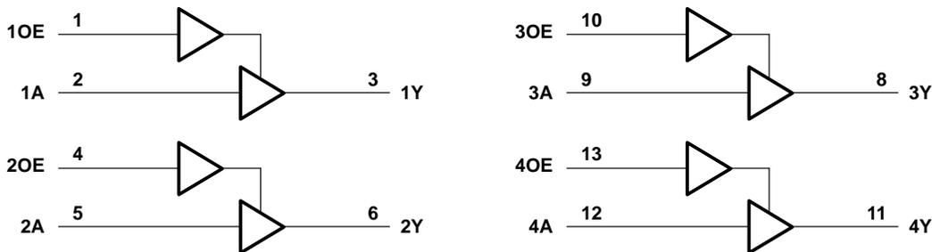
Pin numbers shown are for the D, DB, DGV, J, N, NS, PW, and W packages.
