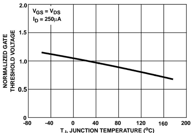
FIGURE 10. NORMALIZED GATE THRESHOLD VOLTAGE vs JUNCTION TEMPERATURE
