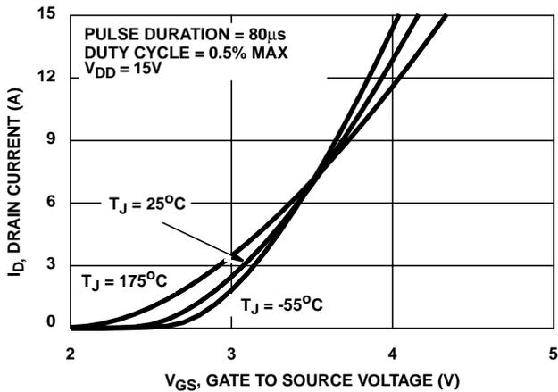
FIGURE 8. TRANSFER CHARACTERISTICS
