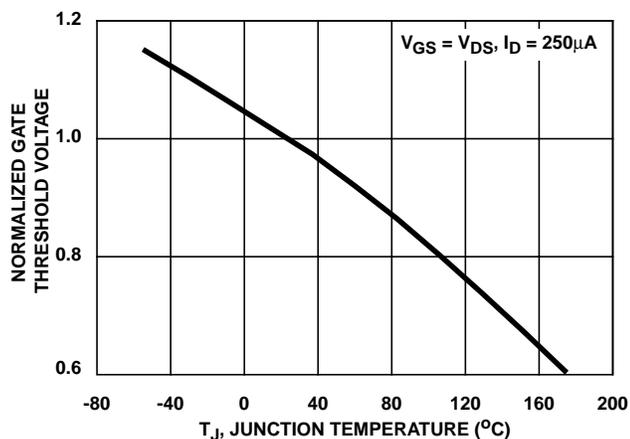
FIGURE 12. NORMALIZED GATE THRESHOLD VOLTAGE vs JUNCTION TEMPERATURE
