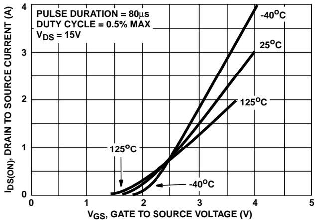
FIGURE 5. TRANSFER CHARACTERISTICS
