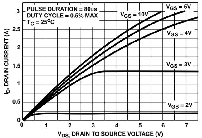
FIGURE 4. SATURATION CHARACTERISTICS
