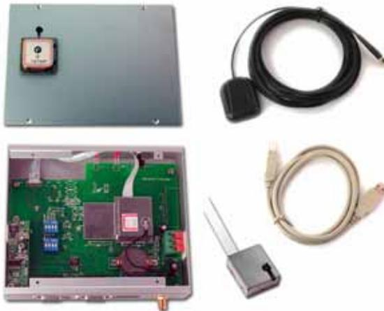
This basic configuration allows dialog between the PC and the evaluation kit using serial communication (COM port) and NMEA character strings provided by and to the PVT module. Based on that NMEA string the GPS Monitor can display position, time, speed, satellite information, position plot and sky plot.
