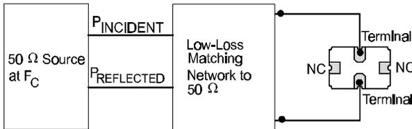
$$CW \text{ RF Power Dissipation} = P_{INCIDENT} - P_{REFLECTED}$$
