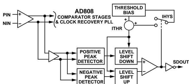
Figure 11. Signal Level Detect Circuit Block Diagram
