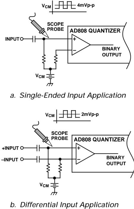
Figure 3. (a–b) Single-Ended and Differential Input Applications
