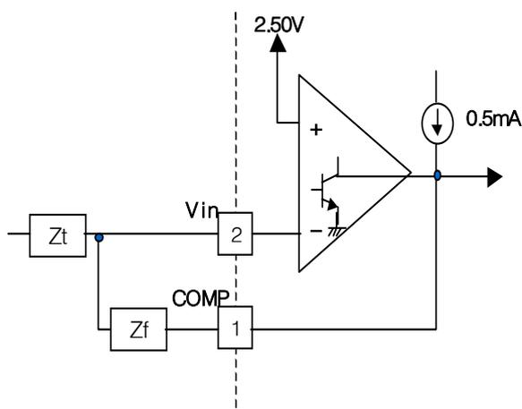
Error amp output(Pin1) is provided for external loop compensation and error amp can source or sink up to 0.5mA. The non-inverting input is internally biased at 2.5V and is not pinned out. The converter output voltage is typically divided down and monitored by the inverting input(pin2).
