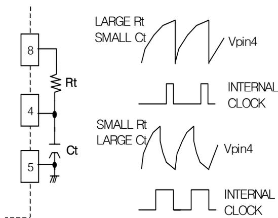
The oscillator frequency is programmed by the values selected for the timing components  $R_t$  and  $C_t$ .  $C_t$  is charged from 5V,  $V_{ref}$ , through resistor  $R_t$  to approximately 2.8V and discharged to 1.2V by an internal current sink.
