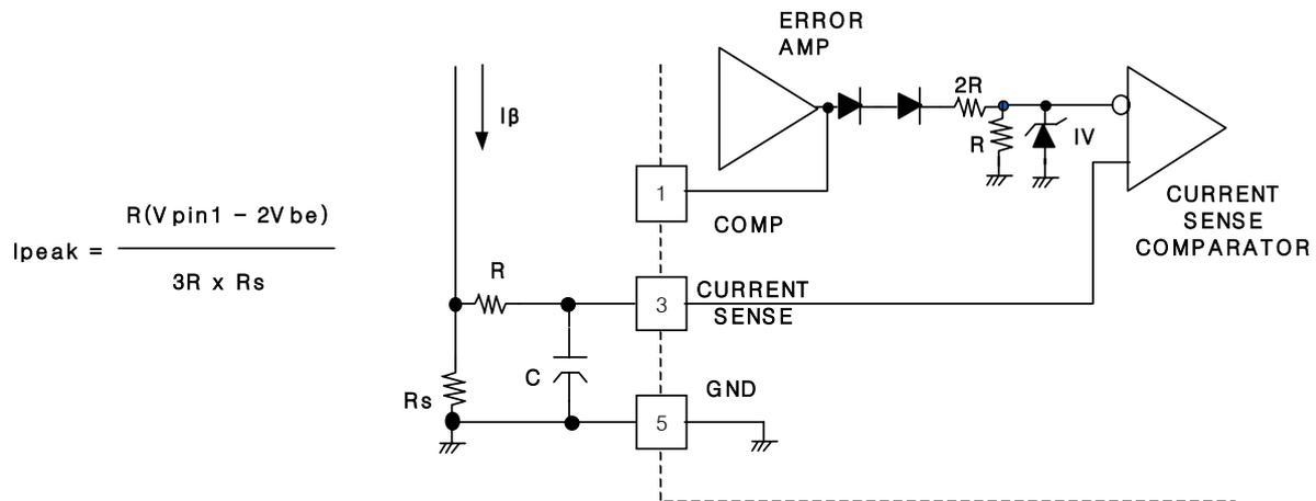
A normal operating conditions occurs when the power supply output is overloaded or if output voltage to 1.0V. Therefore the maximum peak switch current is  $I_{pk(max)} = 1.0V/R_s$ , and under the normal operating conditions the peak inductor current controlled by the voltage at pin1.
