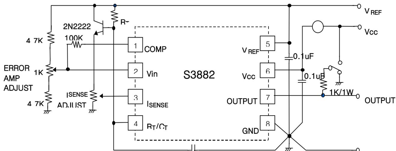
High peak currents associated with capacitive loads necessitate careful grounding techniques. Timing and bypass capacitors should be connected close to Pin5 in a single point ground. The transistor and 5 kΩ potentiometer are used to sample the oscillator waveform and apply an adjustable ramp to Pin 3.
