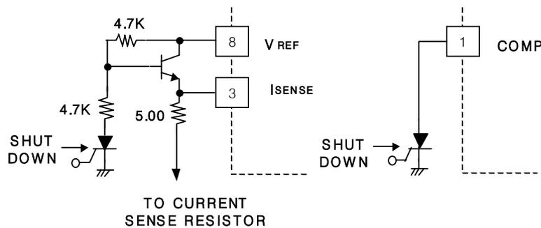
Shutdown of the S3882 can be accomplished by two methods; either raise pin3 above 1V or pull pin1 below a voltage two diodes drops above ground. Either causes the output of the PWM method comparator to be high (refer to
