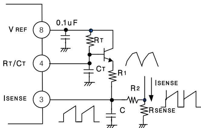
A fraction of the oscillator ramp can be resistively summed with the current sense signal to provide slope compensation for converters requiring duty cycle over 50%. Note that capacitor C, forms a filter with R<sub>2</sub> to suppress the leading edge switch spikes.
