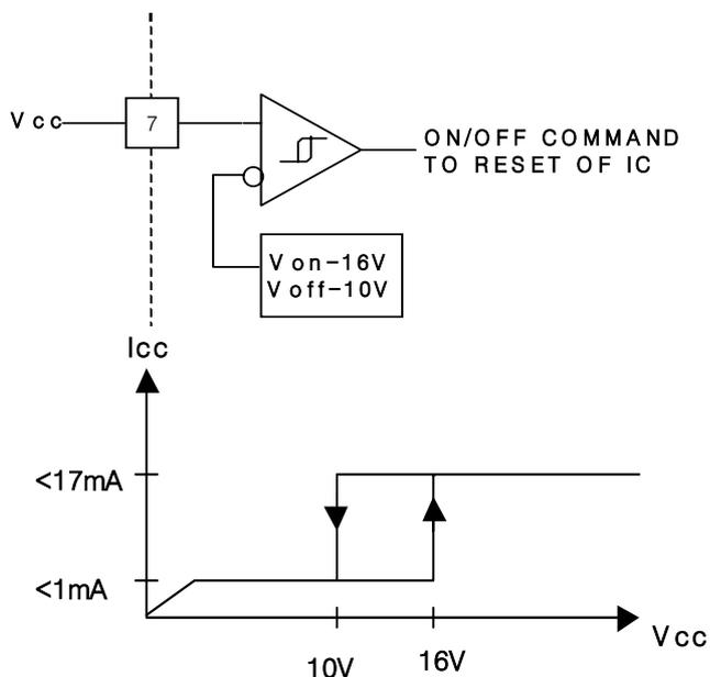
To prevent erratic output behavior which activating the power switch with extraneous leakage currents, during under voltage lockout. Output(pin6) should be shunted to ground with a bleeder resistor.
