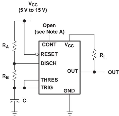
NOTE A: Bypassing the control-voltage input to ground with a capacitor might improve operation. This should be evaluated for individual applications.
