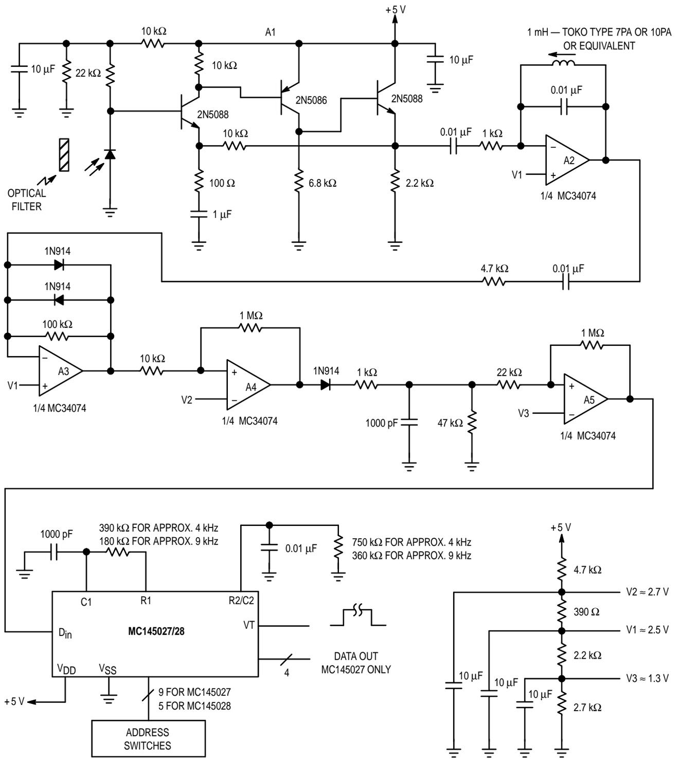
Figure 20. Infrared Receiver
