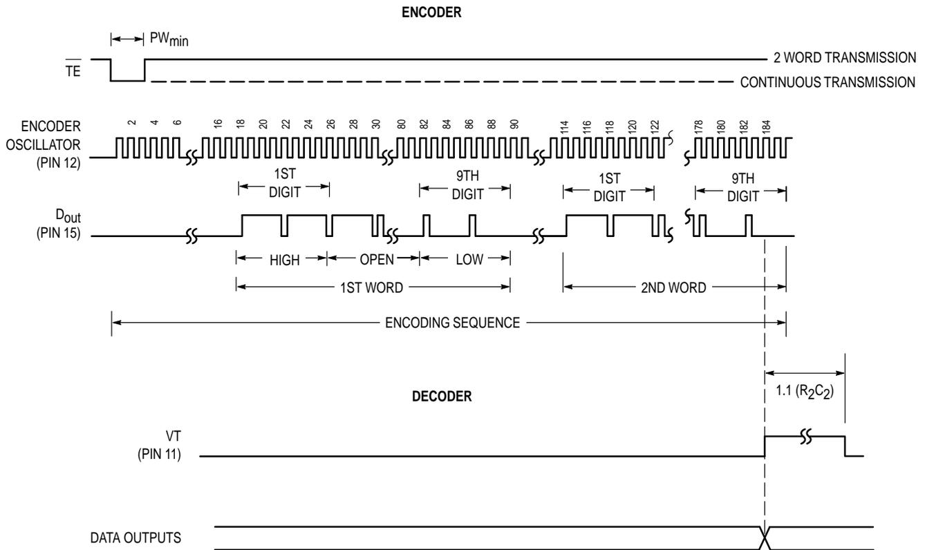
**Figure 10. Timing Diagram**
