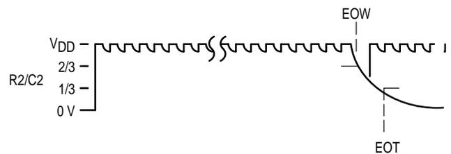
Figure 16. R-C Decay on Pin 10 (R2/C2)
