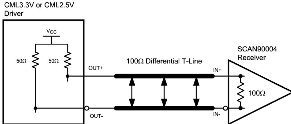
Typical CML Driver DC-Coupled Interface to SCAN90004 Input
