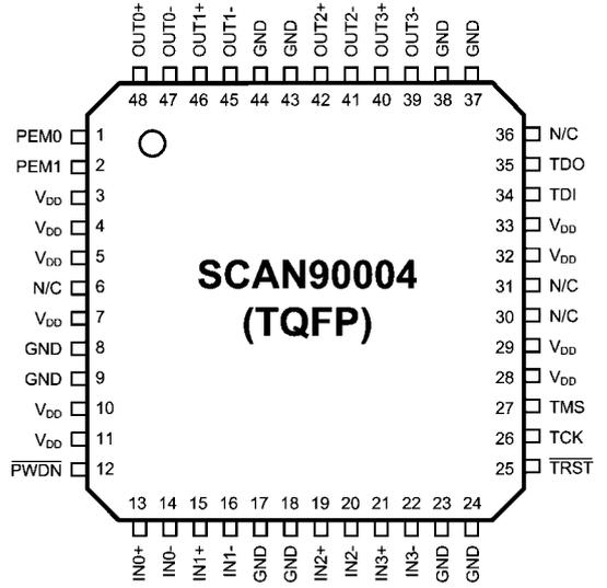
**Pinout - Top View**
