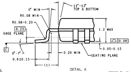
DIMENSIONS ARE IN MILLIMETERS
