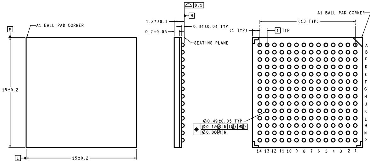
DIMENSIONS ARE IN MILLIMETERS
