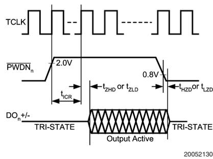
FIGURE 7. Individual Channel Power up Time,  $t_{ICR}$
