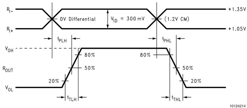
**FIGURE 7. Receiver Propagation Delay and Transition Time Waveforms**
