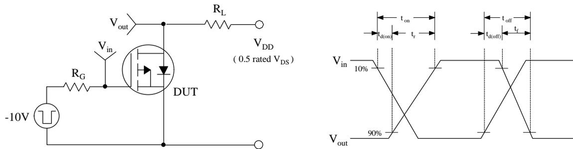
Fig 14. Unclamped Inductive Switching Test Circuit & Waveforms
