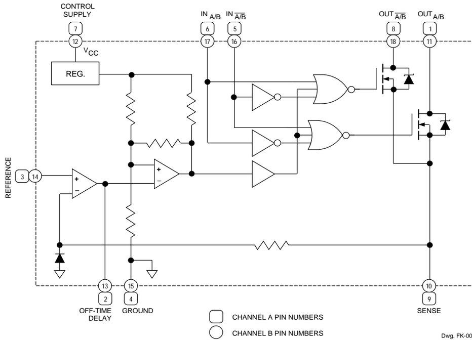
Note that channels A and B are electrically isolated.
