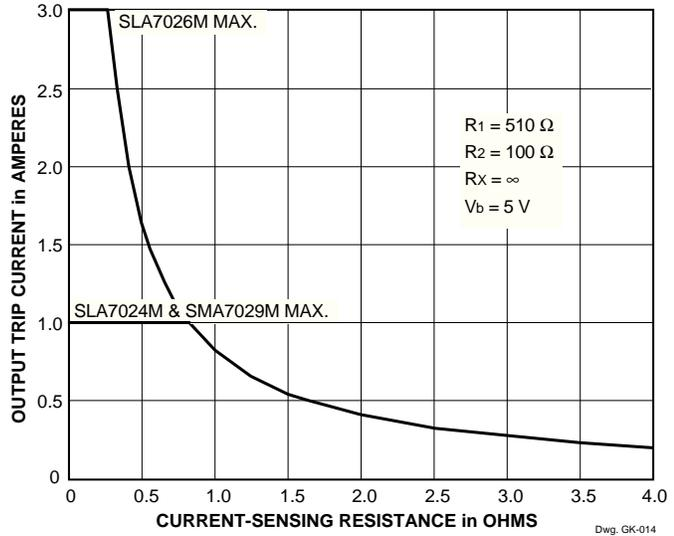
FIGURE 3. CURRENT-SENSING RESISTANCE
