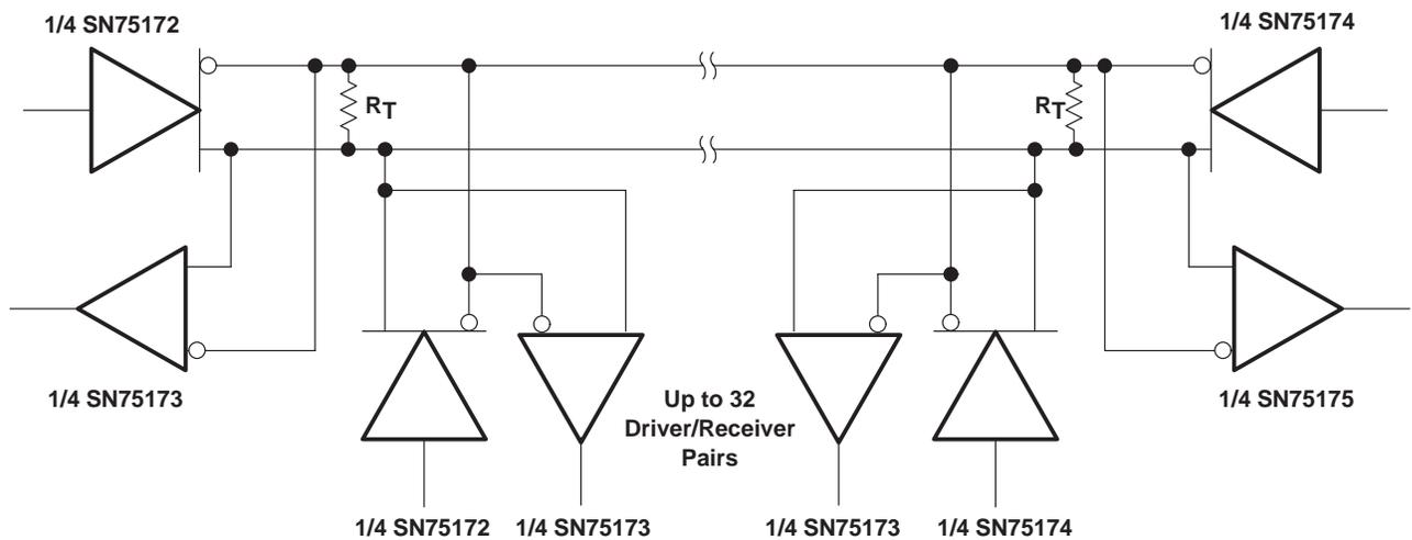
NOTE A: The line should be terminated at both ends in its characteristic impedance ( $R_T = Z_0$ ). Stub lengths off the main line should be kept as short as possible.
