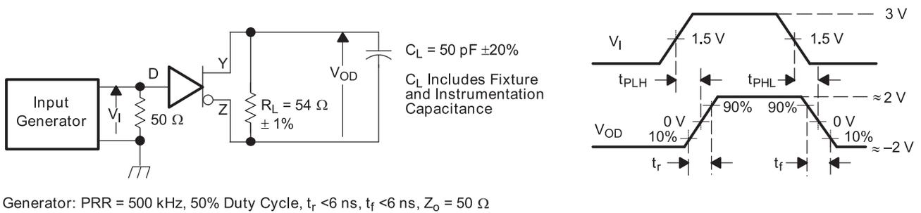
Figure 5. Driver Switching Test Circuit and Voltage Waveforms
