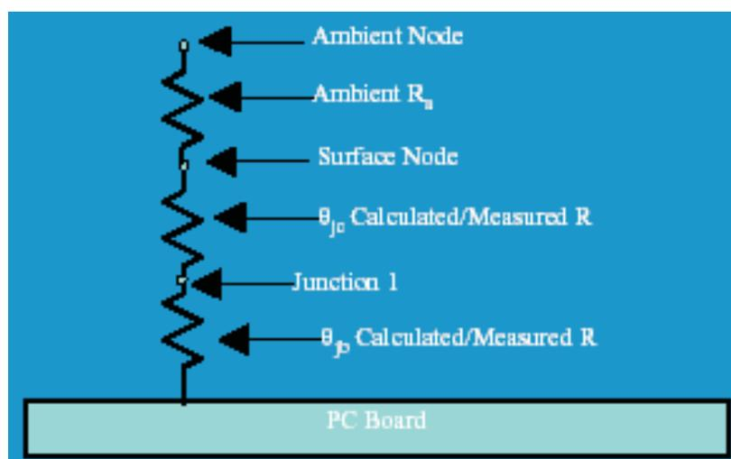
Figure 15. Thermal Resistance
