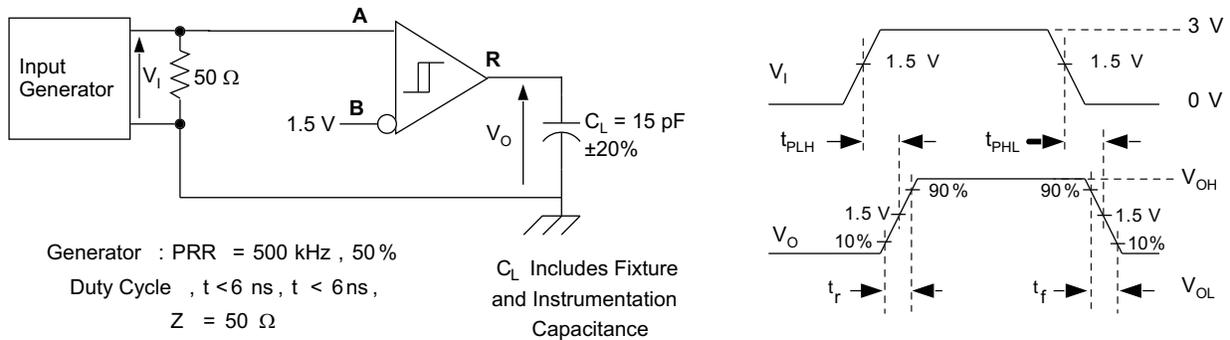
Figure 7. Receiver Switching Test Circuit and Voltage Waveforms
