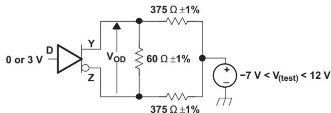
Figure 2. Driver  $V_{OD}$  With Common-Mode Loading Test Circuit
