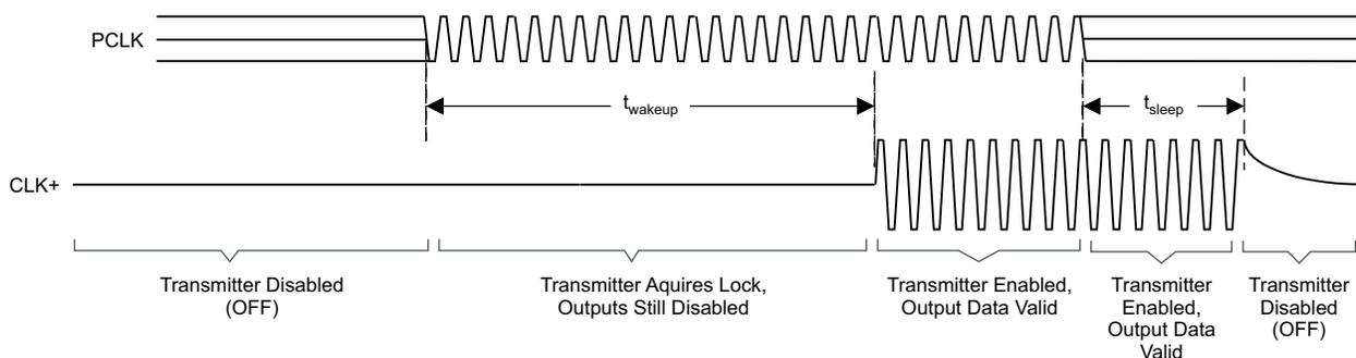
Figure 16. Standby Detection
