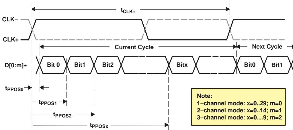
Figure 13.  $t_{SK(0)}$  SubLVDS Output Pulse Position Measurement
