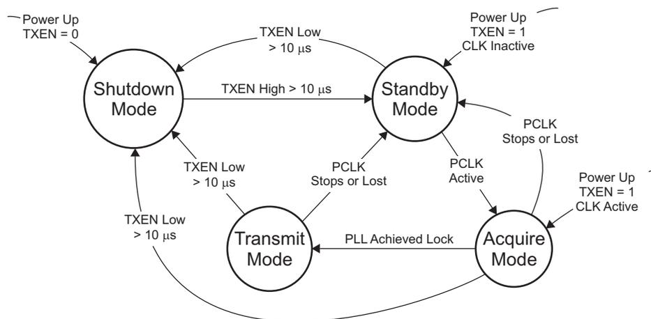
Figure 6. Status Detect and Operating Modes Flow Diagram
