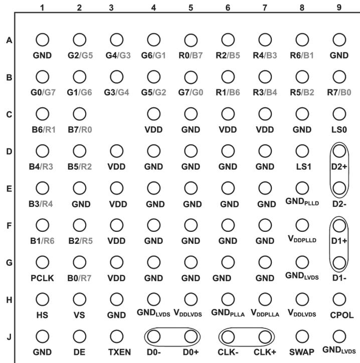
RGB Input pin assignment based on SWAP pin setting:
