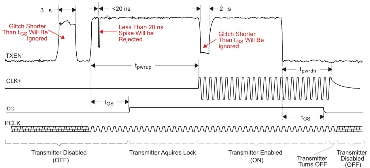
Figure 15. Transmitter Enable Glitch Suppression Time
