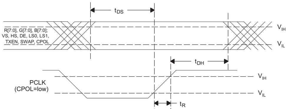
Figure 8. Setup/Hold Time
