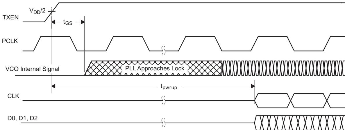
Figure 14. Transmitter Behavior While Approaching Sync
