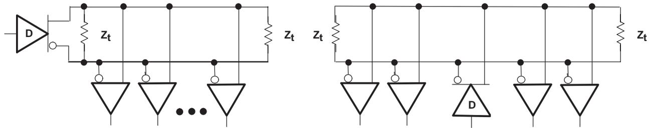
**Figure 18. Multidrop Architectures With Different Driver Locations**
