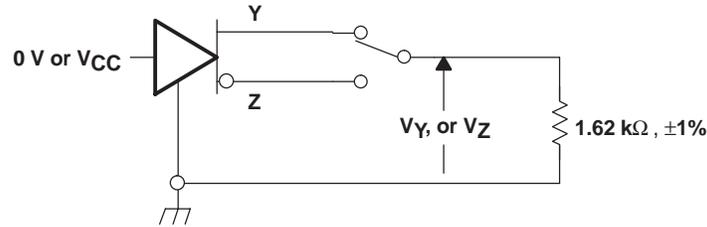
Figure 7. Driver Maximum Steady State Output Voltage
