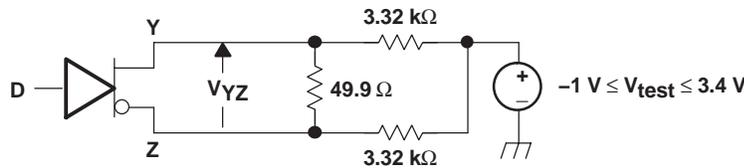
NOTE: All resistors are 1% tolerance.
