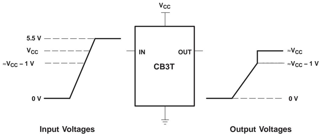
NOTE A: If the input high voltage ( $V_{IH}$ ) level is greater than or equal to  $V_{CC} - 1$  V, and less than or equal to 5.5 V, then the output high voltage ( $V_{OH}$ ) level will be equal to approximately the  $V_{CC}$  voltage level.
