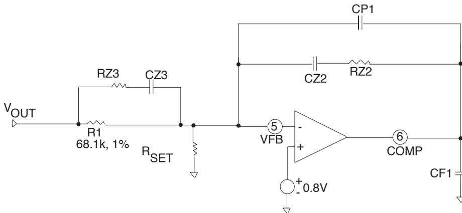
$$R_{SET} = 54.48 / (V_{OUT} - 0.8) \text{ (k}\Omega\text{)}$$
