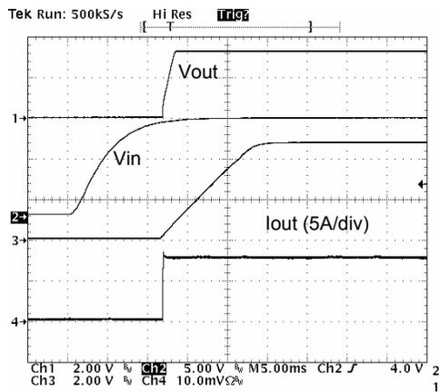
Figure 7. Start-Up Response: 8A Load
