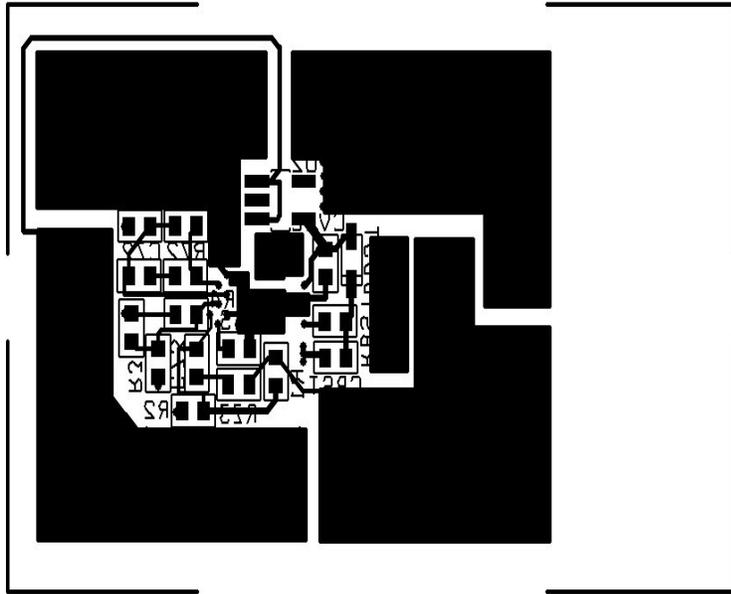
Figure 29. SP7652EB PC Layout Bottom Side
