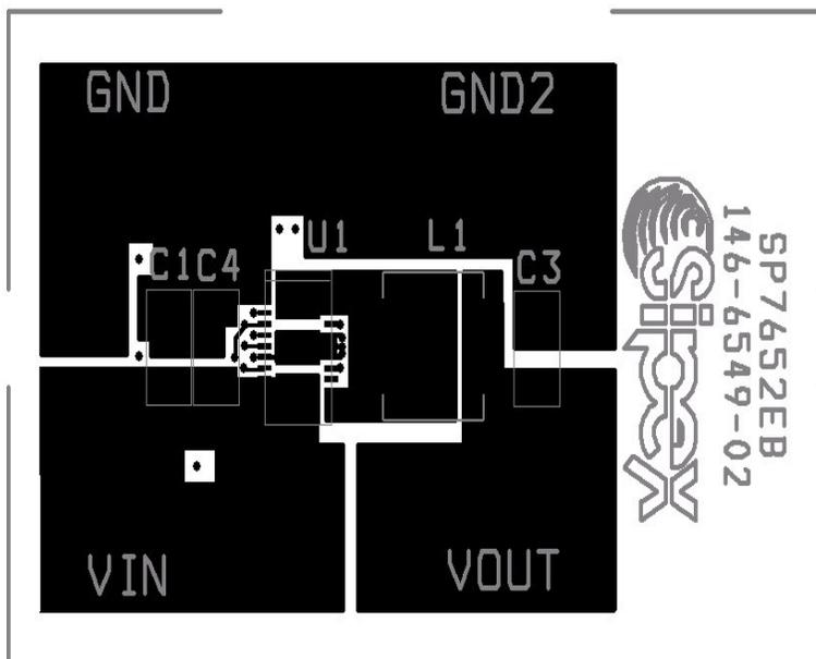
Figure 26. SP7652EB PC Layout Top Side
