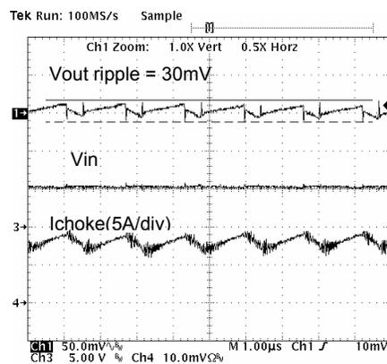
Figure 22. Output Ripple: 8A Load
