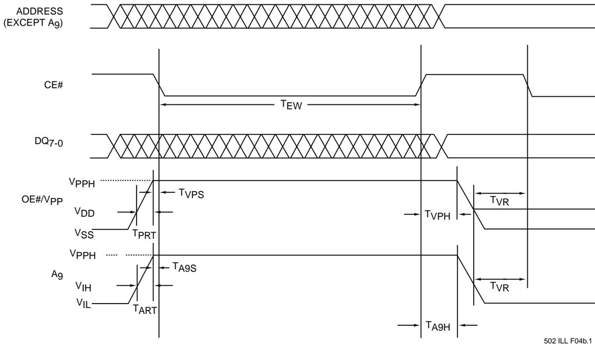
FIGURE 6: READ CYCLE TIMING DIAGRAM FOR SST27SF512
