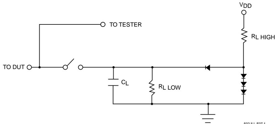
FIGURE 12: A TEST LOAD EXAMPLE
