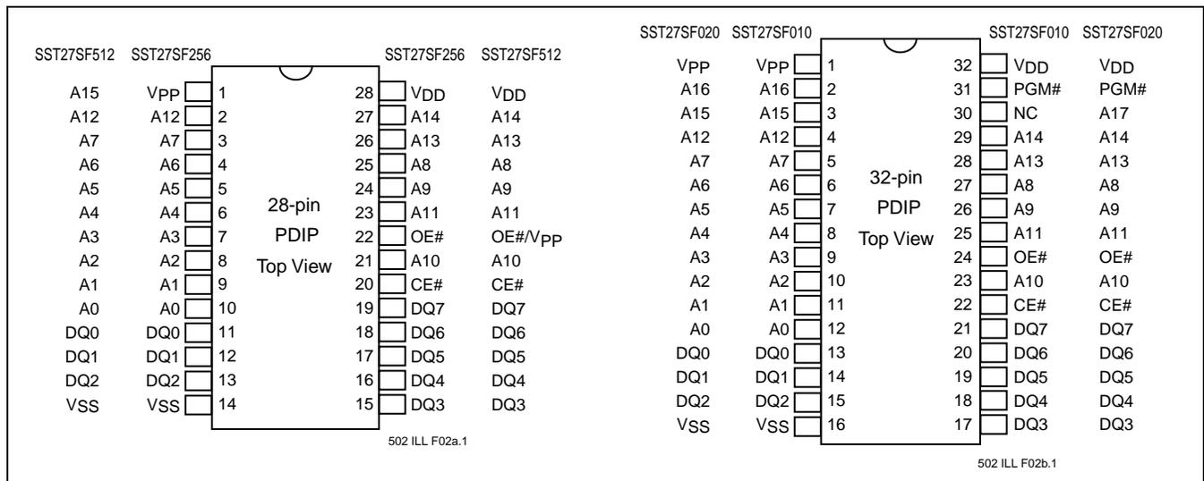
**FIGURE 3: PIN ASSIGNMENTS FOR 28-PIN AND 32-PIN PDIP**
