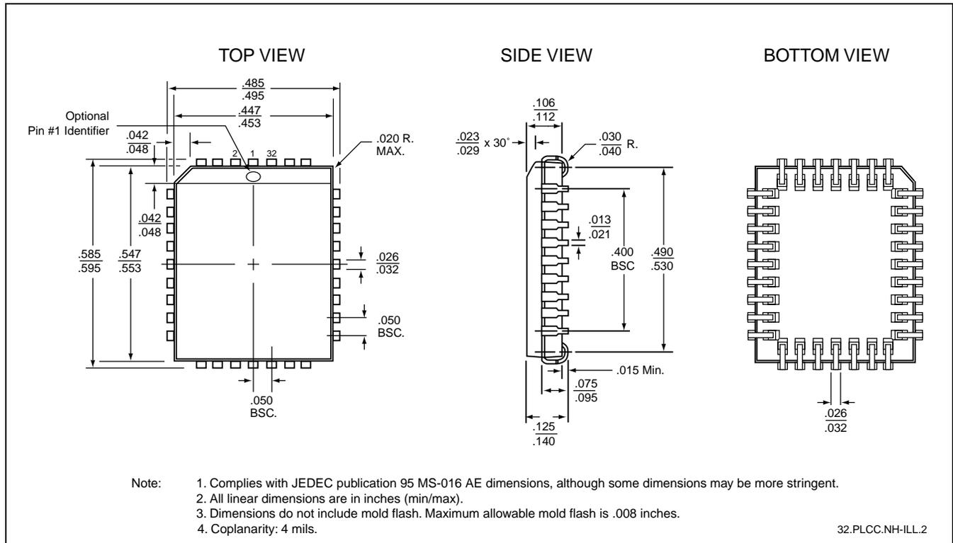
**32-PIN PLASTIC LEAD CHIP CARRIER (PLCC)**
