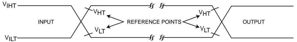
AC test inputs are driven at  $V_{IHT}$  (2.4 V) for a logic "1" and  $V_{ILT}$  (0.4 V) for a logic "0". Measurement reference points for inputs and outputs are  $V_{HT}$  (2.0 V) and  $V_{LT}$  (0.8 V). Input rise and fall times (10%  $\leftrightarrow$  90%) are <10 ns.
