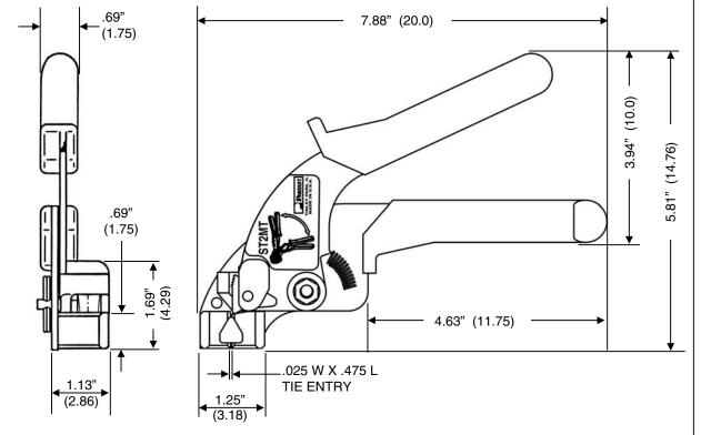
NOTES, UNLESS OTHERWISE SPECIFIED: PANDUIT TOOL NUMBER ST2MT IS USED TO INSTALL ALL STANDARD, LIGHT-HEAVY, HEAVY AND EXTRA-HEAVY CROSS SECTION PAN-STEEL TYPE MLT TIES, TYPE MLTC COATED TIES AND TYPE MLTDH DOUBLE WRAPPED TIES.
