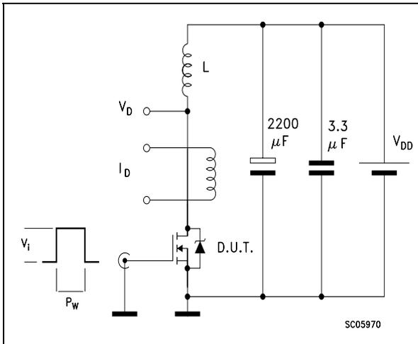
Figure 20: Switching Times Test Circuit For Resistive Load
