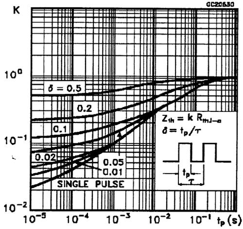
Thermal Impedance For ISOWATT218
