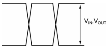
Figure 1a. Single-Ended Voltage Swing
