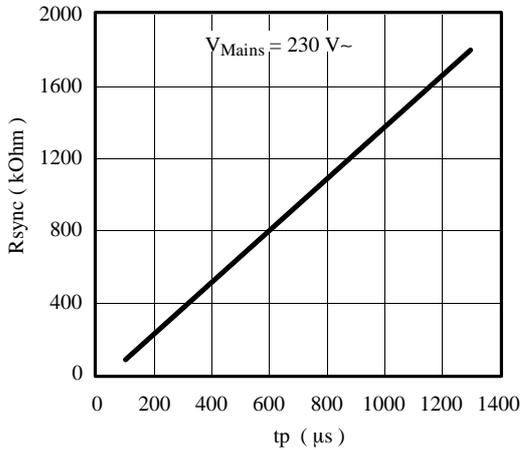
Figure 6. Synchronization resistance
