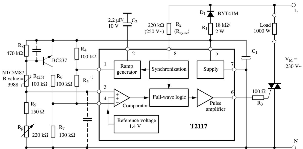
Figure 11. Temperature control 15 to 35°C with sensor monitoring
