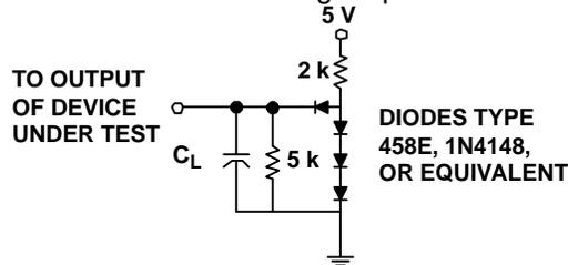
C<sub>L</sub> includes test-fixture and probe capacitance.
