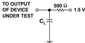
C<sub>L</sub> includes test-fixture and probe capacitance.
