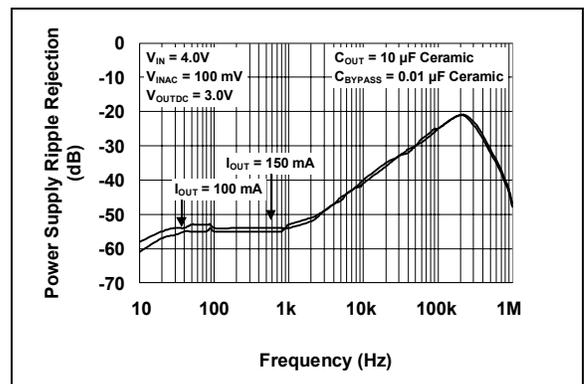
**FIGURE 2-24:** PSRR vs. Frequency ( $C_{OUT} = 10 \mu F$  Ceramic).
