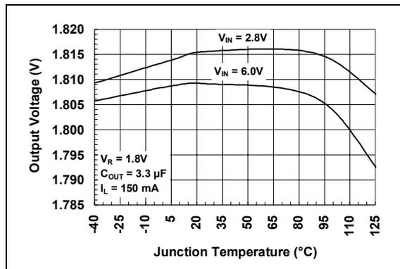
**FIGURE 2-4:** Output Voltage vs. Junction Temperature (150 mA).
