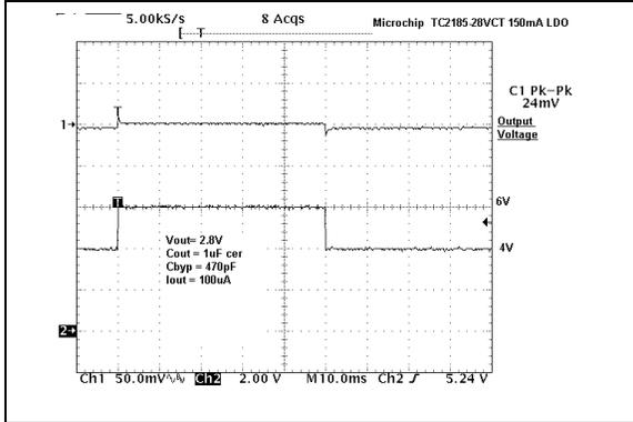
**FIGURE 2-19:** Line Transient Response. ( $C_{OUT} = 1 \mu F$ ).
