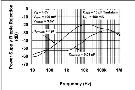
FIGURE 2-25: PSRR vs. Frequency ( $C_{OUT} = 10 \mu F$  Tantalum).
