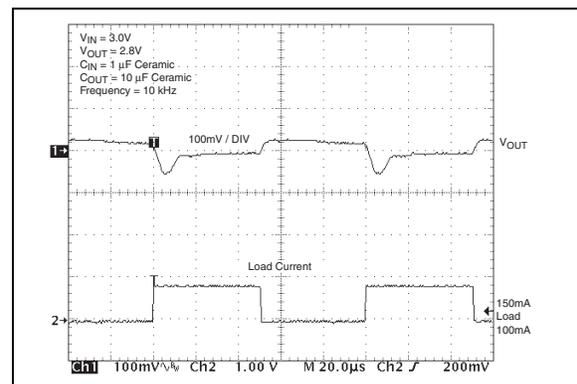
**FIGURE 2-18:** Load Transient Response. ( $C_{OUT} = 10 \mu F$ ).
