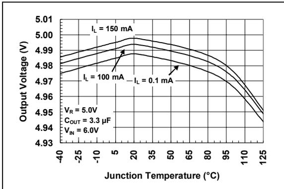
**FIGURE 2-14:** Output Voltage vs. Junction Temperature (150 mA).
