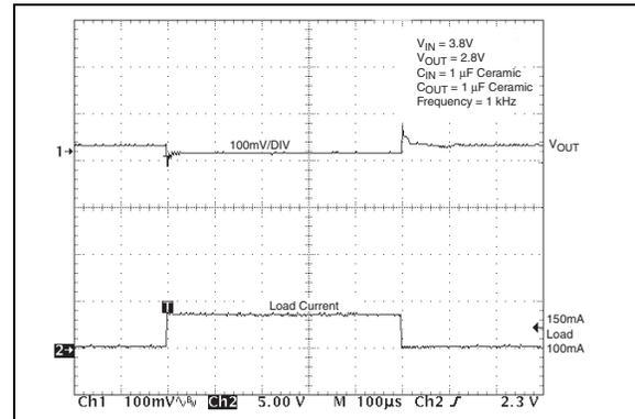
**FIGURE 2-17:** Load Transient Response. ( $C_{OUT} = 1 \mu F$ ).
