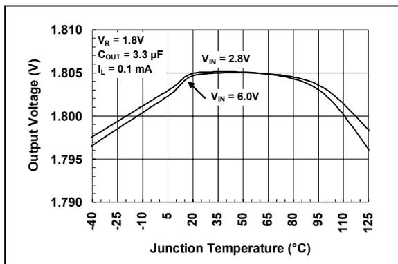
**FIGURE 2-3:** Output Voltage vs. Junction Temperature (0.1 mA).
