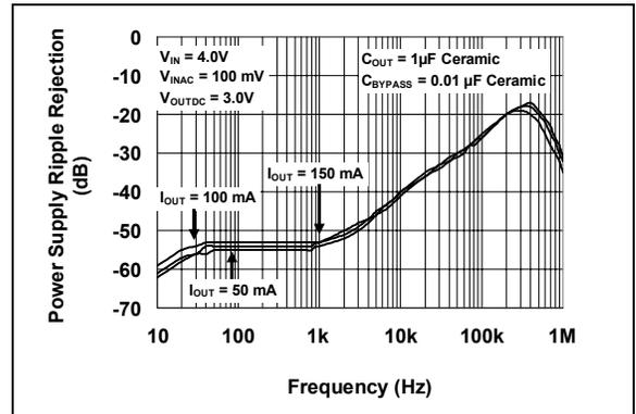
**FIGURE 2-23:** PSRR vs. Frequency ( $C_{OUT} = 1 \mu F$  Ceramic).
