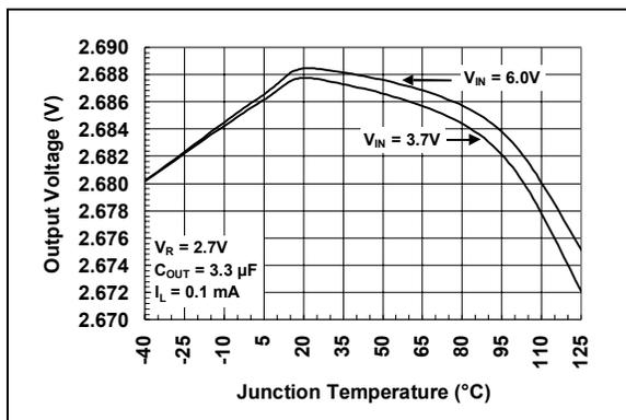
**FIGURE 2-9:** Output Voltage vs. Junction Temperature (0.1 mA).
