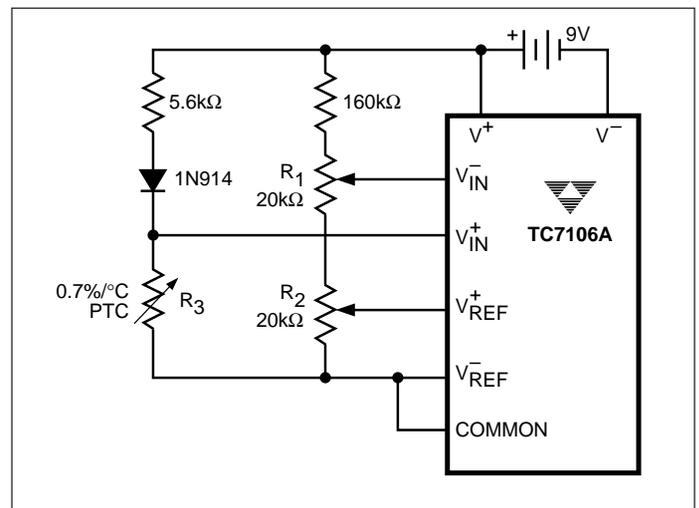
Figure 20. Positive Temperature Coefficient Resistor Temperature Sensor
