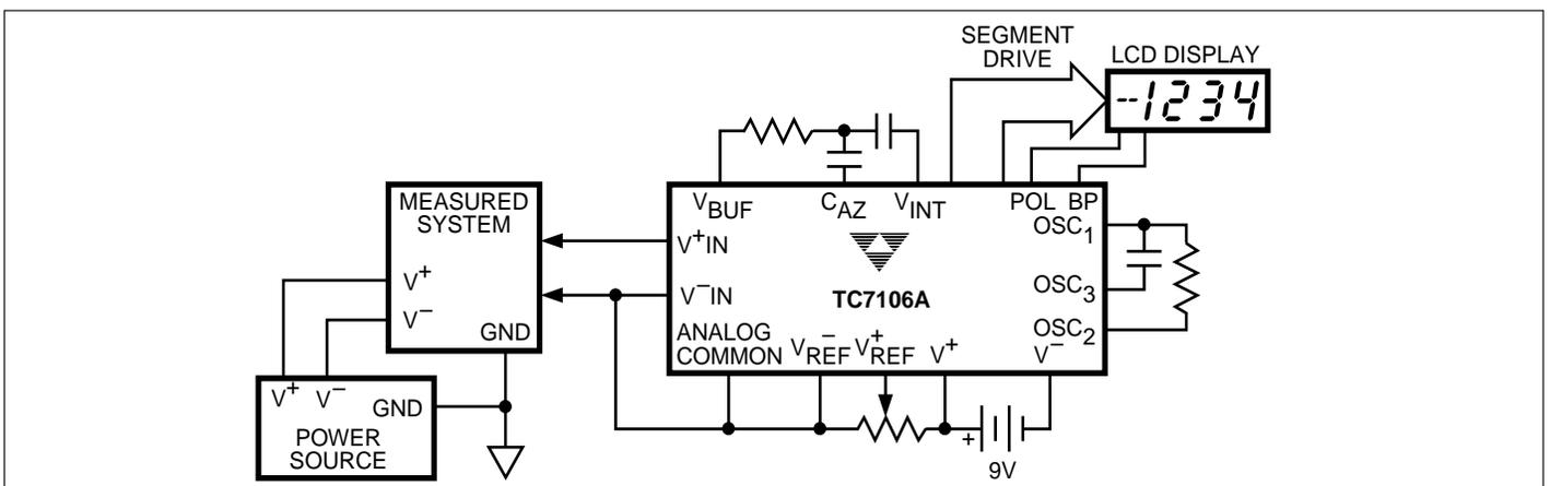
Figure 8. Common-Mode Voltage Removed in Battery Operation with  $V_{\text{CM}} = \text{Analog Common}$
