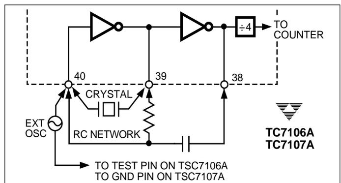
Figure 6. Clock Circuits
