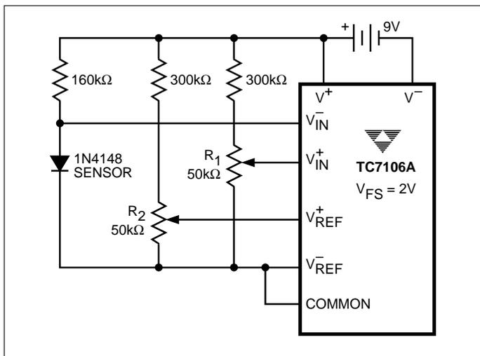
Figure 19. Temperature Sensor
