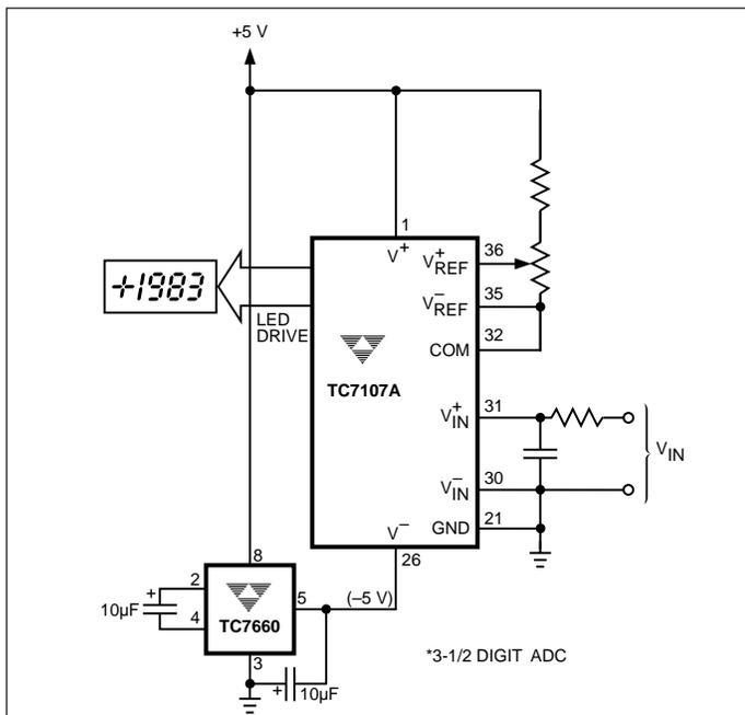
Figure 13. Negative Power Supply Generation with TC7660
