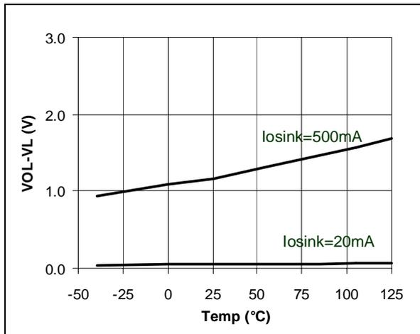
Figure 10: High level output voltage vs temp.
