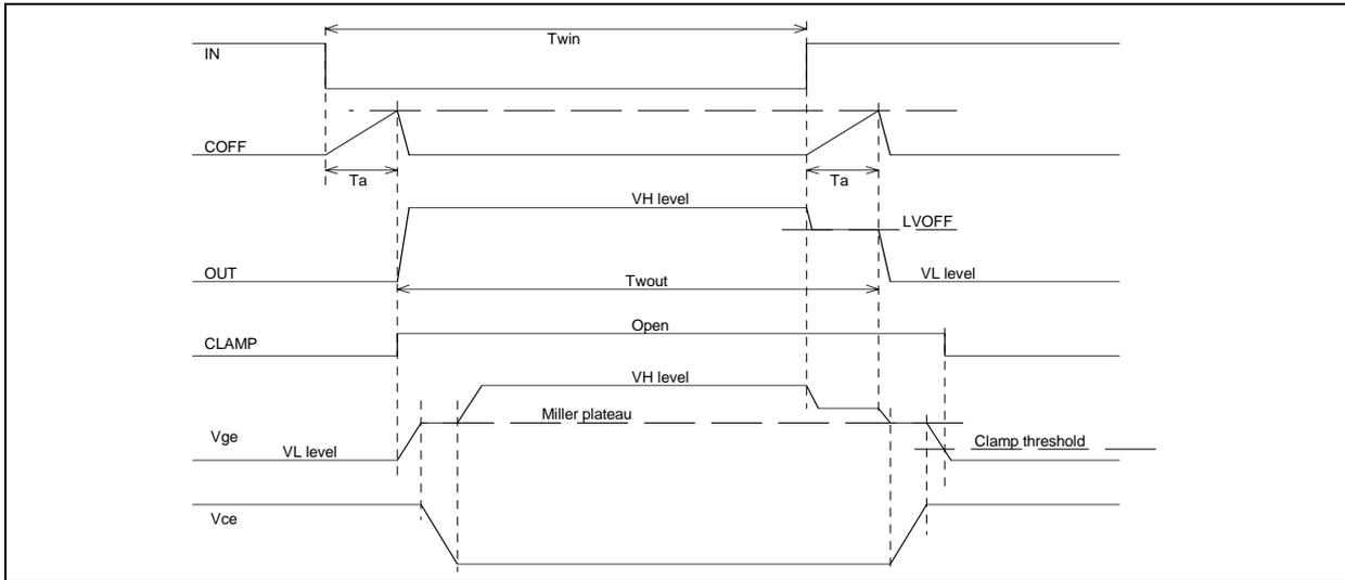
Figure 4: input and output waveform dynamic parameters
