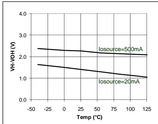
Figure 8: Sink current vs temperature
