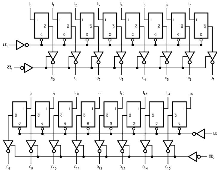
Please note that these diagrams are provided only for the understanding of logic operations and should not be used to estimate propagation delays.
