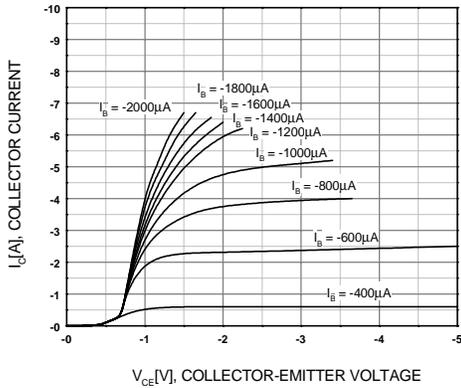
Figure 1. Static Characteristic
