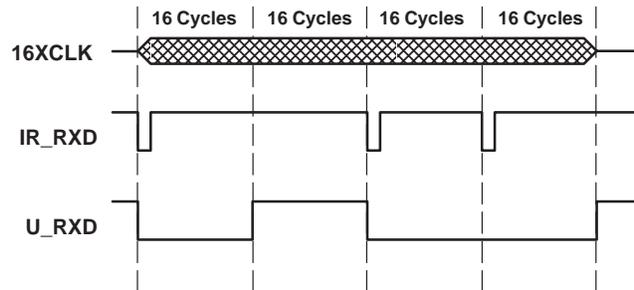
Figure 5. Decoding Scheme – Macro View
