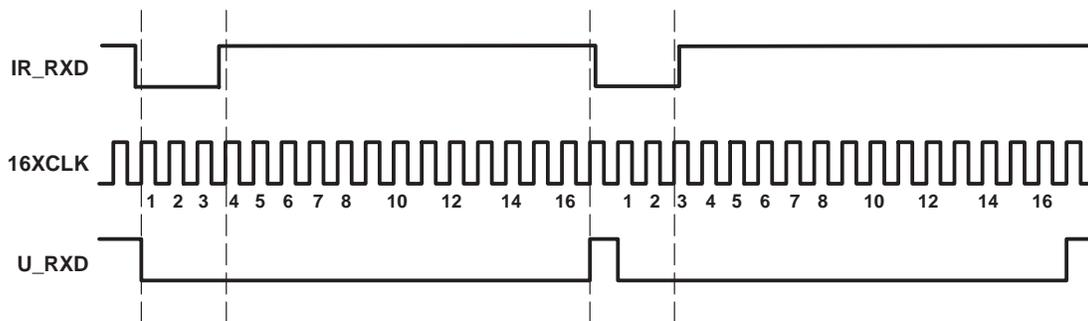
Figure 6. Timing Causing 1-clock-wide Pulse Between Consecutive Ones
