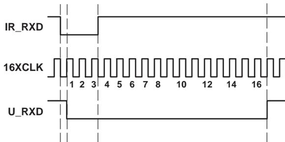
Figure 4. IrDA-SIR Decoding Scheme – Detailed Timing Diagram
