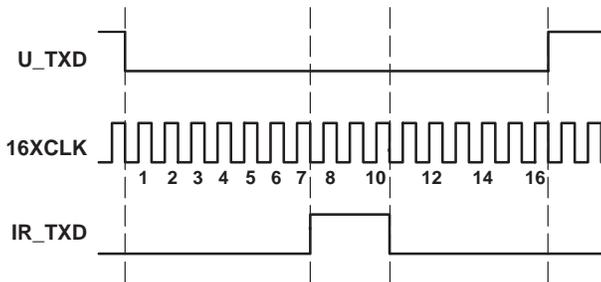
Figure 2. IrDA-SIR Encoding Scheme – Detailed Timing Diagram
