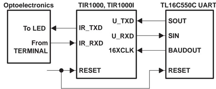
Figure 1. Typical application of the TIR1000, TIR1000I
