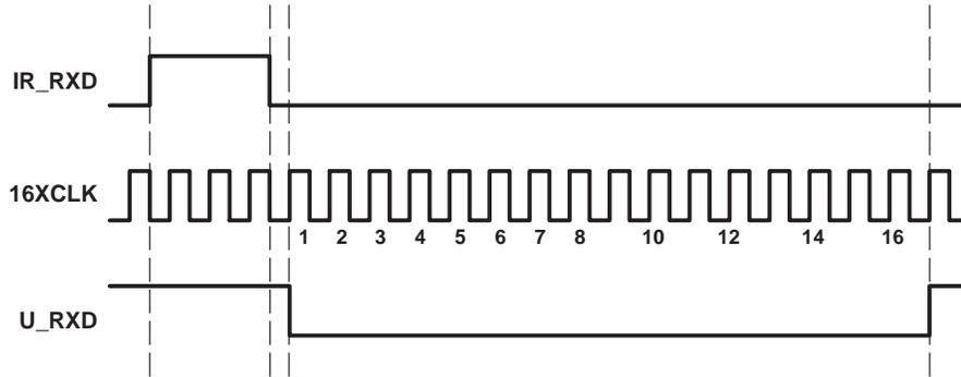
Figure 8. Positive IR\_RXD Pulse Decode – Detailed View
