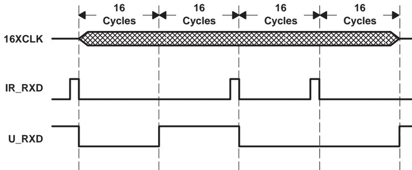
Figure 9. Positive IR\_RXD Pulse Decode – Macro View
