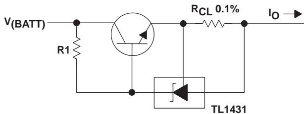
$$I_O = \frac{V_{I(\text{ref})}}{R_{CL}} + I_{KA}$$
