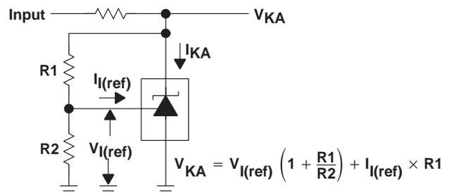
Figure 2. Test Circuit for  $V_{(KA)} > V_{\text{ref}}$
