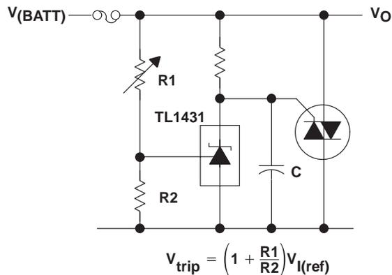
NOTE A: Refer to the stability boundary conditions in Figure 15 to determine allowable values for C.
