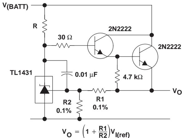
NOTE A: R should provide cathode current  $\geq 1$  mA to the TL1431 at minimum  $V(\text{BATT})$ .
