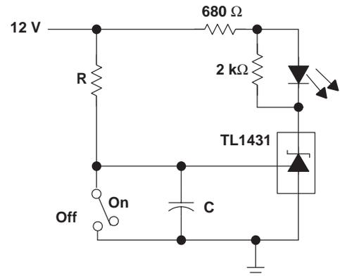
$$\text{Delay} = R \times C \times I_{I(12V)} \frac{12V}{12V - V_{I(\text{ref})}}$$
