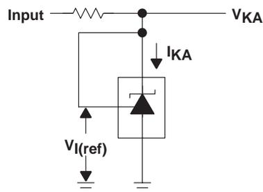
Figure 1. Test Circuit for  $V_{(KA)} = V_{\text{ref}}$
