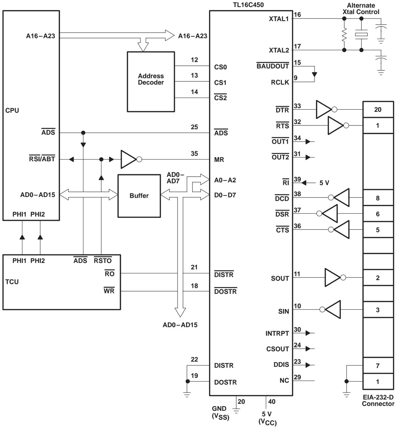
Figure 9. Typical TL16C450 Connection to a CPU
