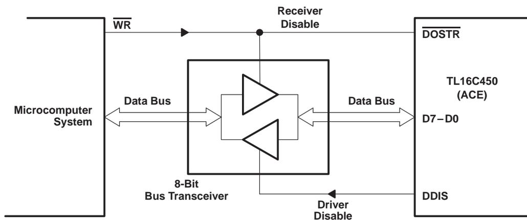
Figure 8. Typical Interface for a High-Capacity Data Bus
